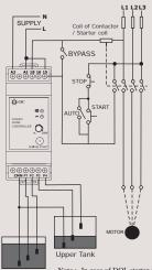
ver Tank Note :- In case of DOL starter connection with LLC, Connect 15 & 18 nos of Liquid level controller to 93 & 95 nos. of DOL Starter respectively
